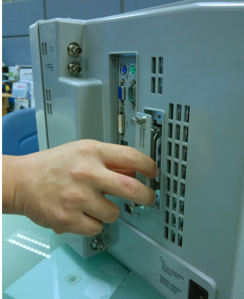
Figure 3-7 Pull and remove the hard drive from the slot
