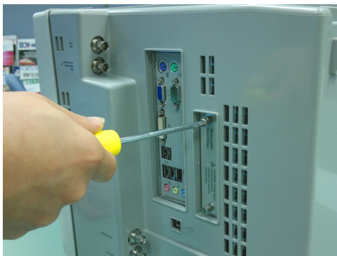
Figure 3-6 Unscrew the hard drive
